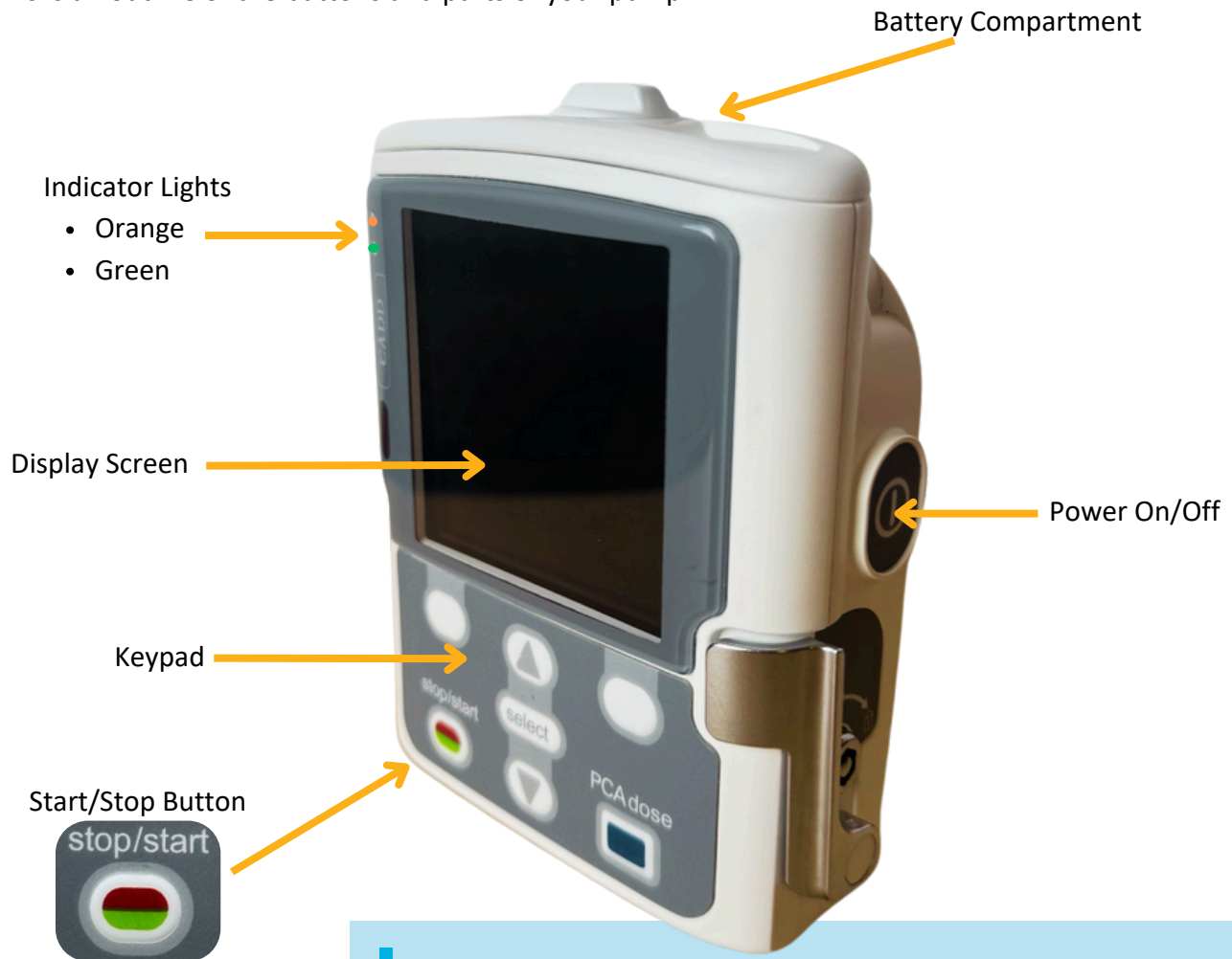
Photo 1: Main parts of the pump - indicator lights, front display, top battery compartment, and keypad with start/stop button.
